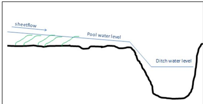
Figure 7: Diagram of hypothetical water surface profile within Agassiz Pool during periods of sheet flow.
