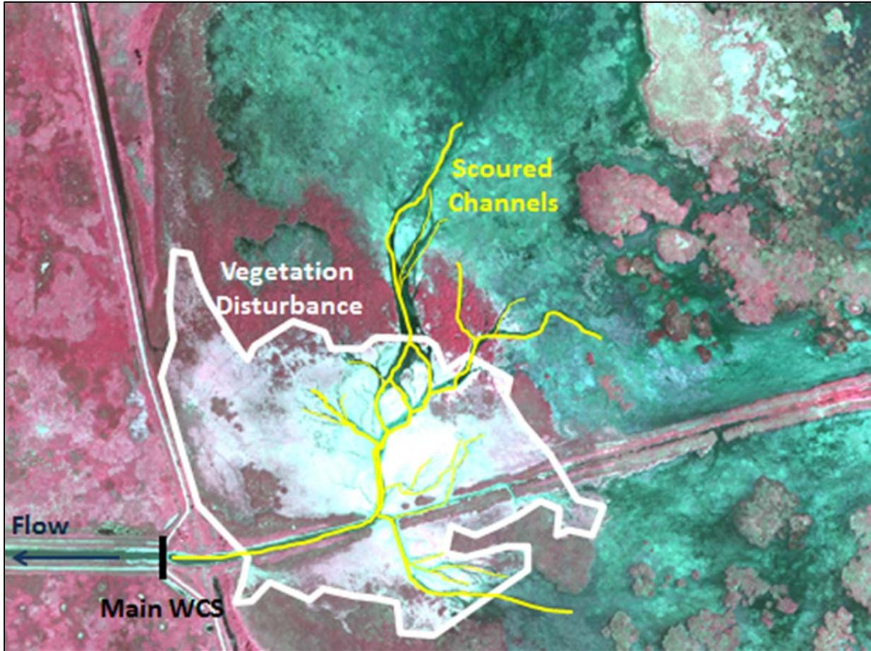
Figure 6: USFWS infrared imagery of Agassiz Pool and the Main WCS on August 7, 2012 approximately 7 days after the radial gates were opened to initiate a drawdown of the Pool. Areas of flattened and/or scoured vegetation are evident along with channels eroded through the wetland substrate.
