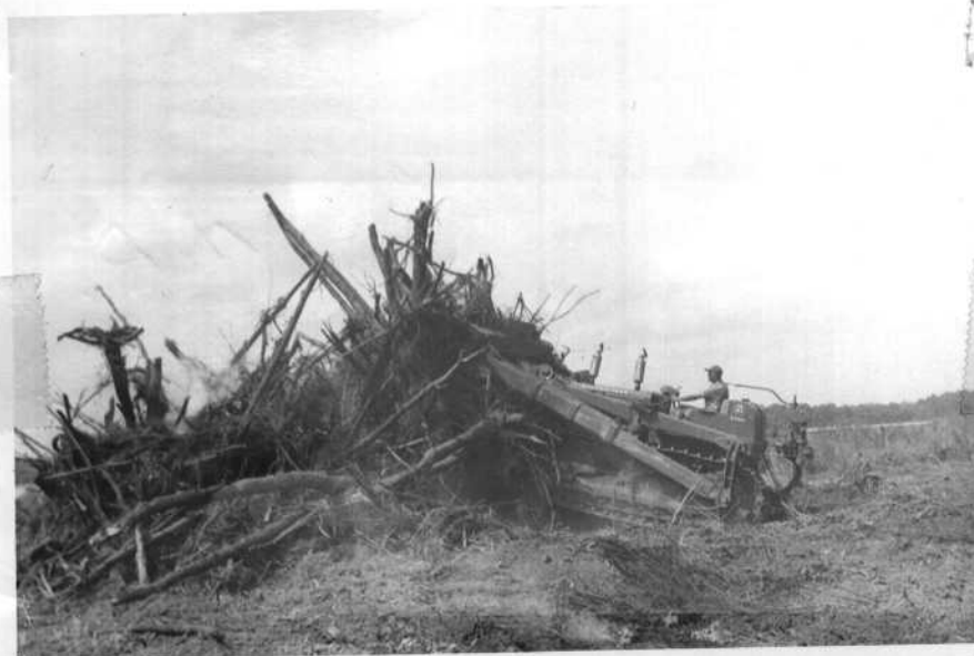
No. 2. Td-18 pushing in for second burning of brush pile hedgerow clearing, River bank fields, Garth Slough.
