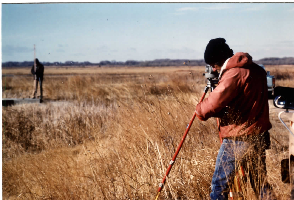
Figure 28. Regional Surveyor Pat Carson spent several days on the refuge surveying the water control structures to allow the collection for capacity information to be used to prove up on our water right. 89-DH
