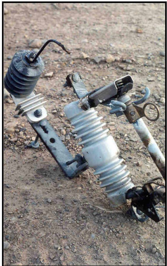
Photo 20 Damaged Cutout Resulting from an Animal Contact
