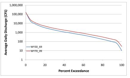
Figure 28. Flow duration curves of average daily discharge in the Grand River near Sumner, MO for Water Years 1930-69 and 1970-2009 for USGS gauge #06902000.
