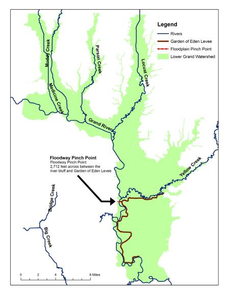
Figure 22. Constriction pinch point in the Grand River floodway caused by the Garden of Eden levee.
