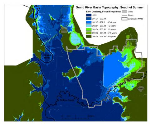
Figure 13. Flood frequency elevation contours south of Sumner, MO.
