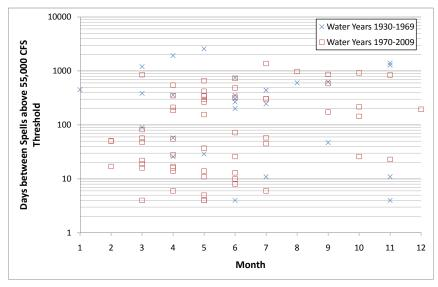
Figure 29. Occurrence of events with average daily discharge in the Grand River near Sumner, MO in excess of 55,000 cfs, shown by month for Water Years 1930-69 and 1970-2009 for USGS gauge #06902000.
