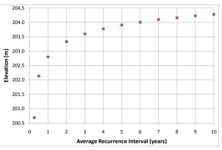
Figure 12. River elevation vs. recurrence interval for the Grand River near Sumner, MO based on peak over threshold analysis of average daily discharge for Water Years 1925-2009 and 3/15/2010 rating table for USGS gauge #06902000.
