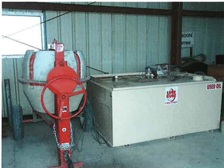
Fig.25 The new concrete mixer and doubled-walled used oil tank.
