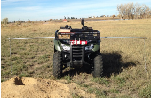
Figure 1. Three meter pole attached at midpoint to ATV
