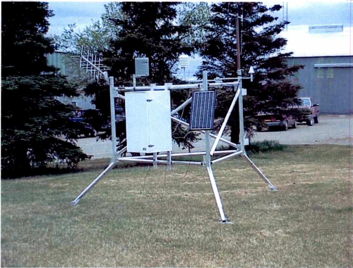
Forest Technology Systems Remote Area Weather Station (RAWS) set up in FWS compound King Salmon for testing.
