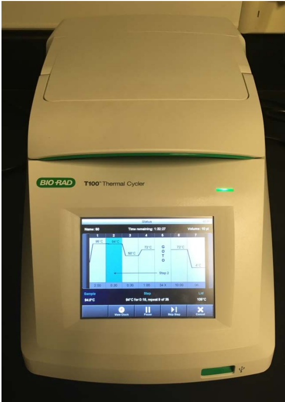
The instrument is a Bio-Rad T100 Thermal Cycler, which is used for conducting polymerase chain reactions (PCR) for amplifying DNA. Photo by David Berg.
