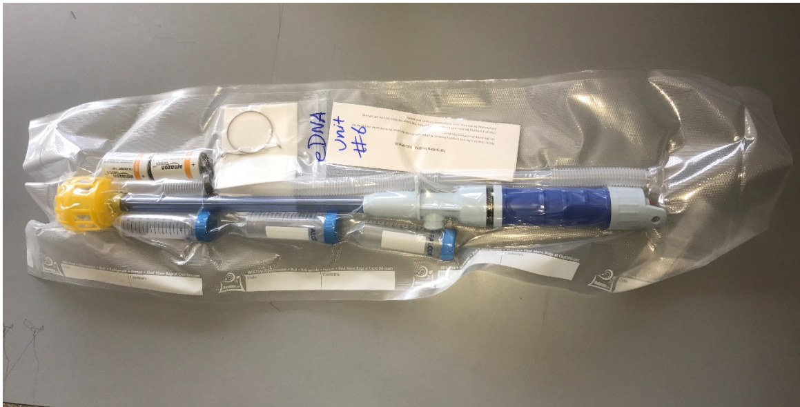
eDNA sampling kit designed to use for this project. Kit consists of a battery operated hand pump, tubing, filters, and collection tubes for storage of filters. (Photo credit: David Hayes - EKU)
