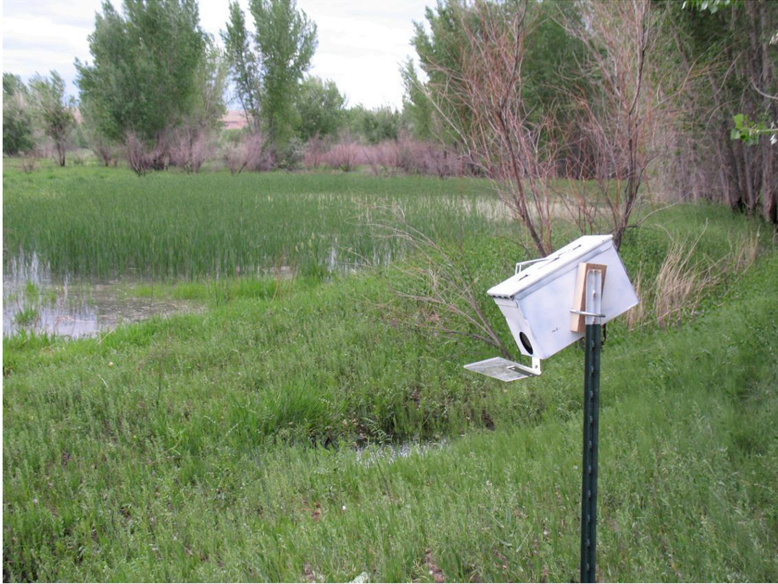
**Figure 2.** Anabat ultrasonic bat detectors were fitted inside metal cases and affixed to steel posts. Detector microphones were oriented downward to avoid damage from weather. Bat calls were deflected into the microphone from an acrylic glass plate mounted on a steel bracket near the bottom of the case. These detectors were programmed to automatically turn on and off near sunset and sunrise.
