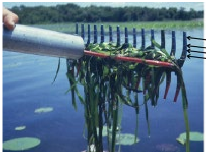
Figure 5. Rake sampler used to sample aquatic vegetation in turbid-water units (photo from Yen and Kreiling 2011). Arrows show the lines used to indicate increments used to estimate total plant density. Vegetation hanging from the rake teeth would be added to the rake before estimating total SAV density.
