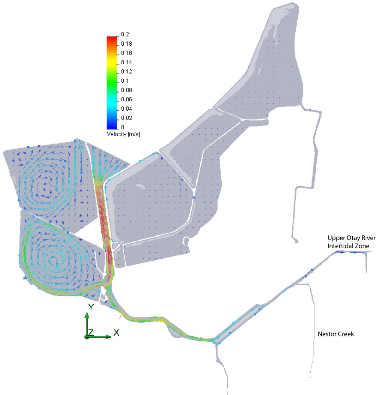
Figure 2: Hydrodynamic simulation of progressive vector flow distribution at 30 min time integration during maximum flood flow during spring tides for the existing lower Otay River and salt pond system based on 2011 WRA bathymetric survey and the 1983-2001 tidal epoch for San Diego Bay tides.
