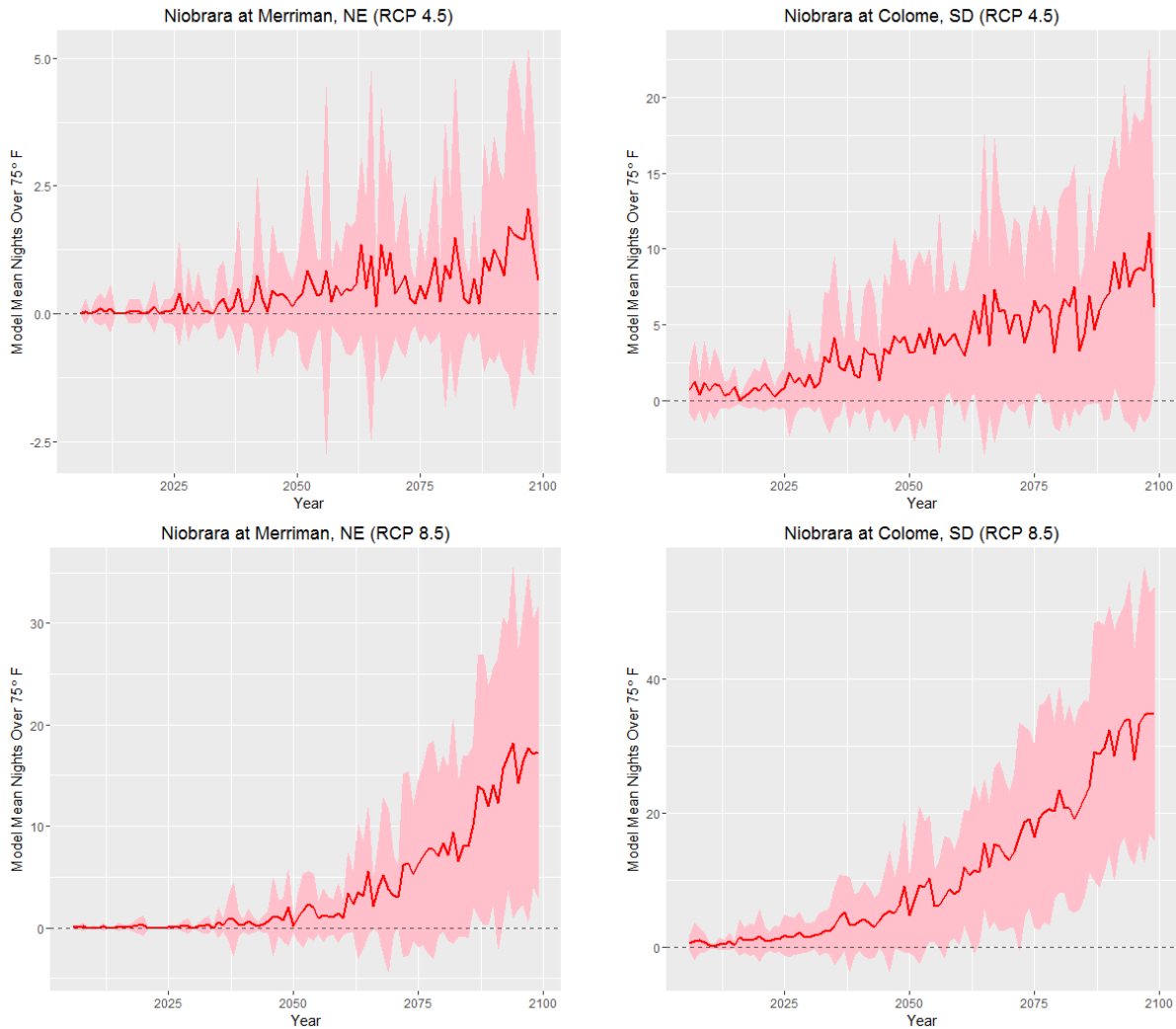
Figure A. The mean (red line) and standard deviation (pink shading) of 20 statistically downscaled climate change models for two locations (East = Colome, SD; West = Merriman, NE) within the Niobrara Analysis Area. Each graph shows the change over time in the mean number of nights with minimum temperatures greater than or equal to 75°F. American Burying Beetles in captivity cannot reproduce when temperatures exceed 75°F.
