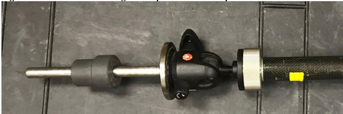
**Parts of the adapter.** We calculated the height of the GNSS antenna when attached to the USGS Fixed-Dimension Adapter (Figure 1) using methods from the national geodetic survey (NOAA, Undated Report). Due to differences between the old and new adapters, Measurements 2, 3, and 4 need to be recalculated.
