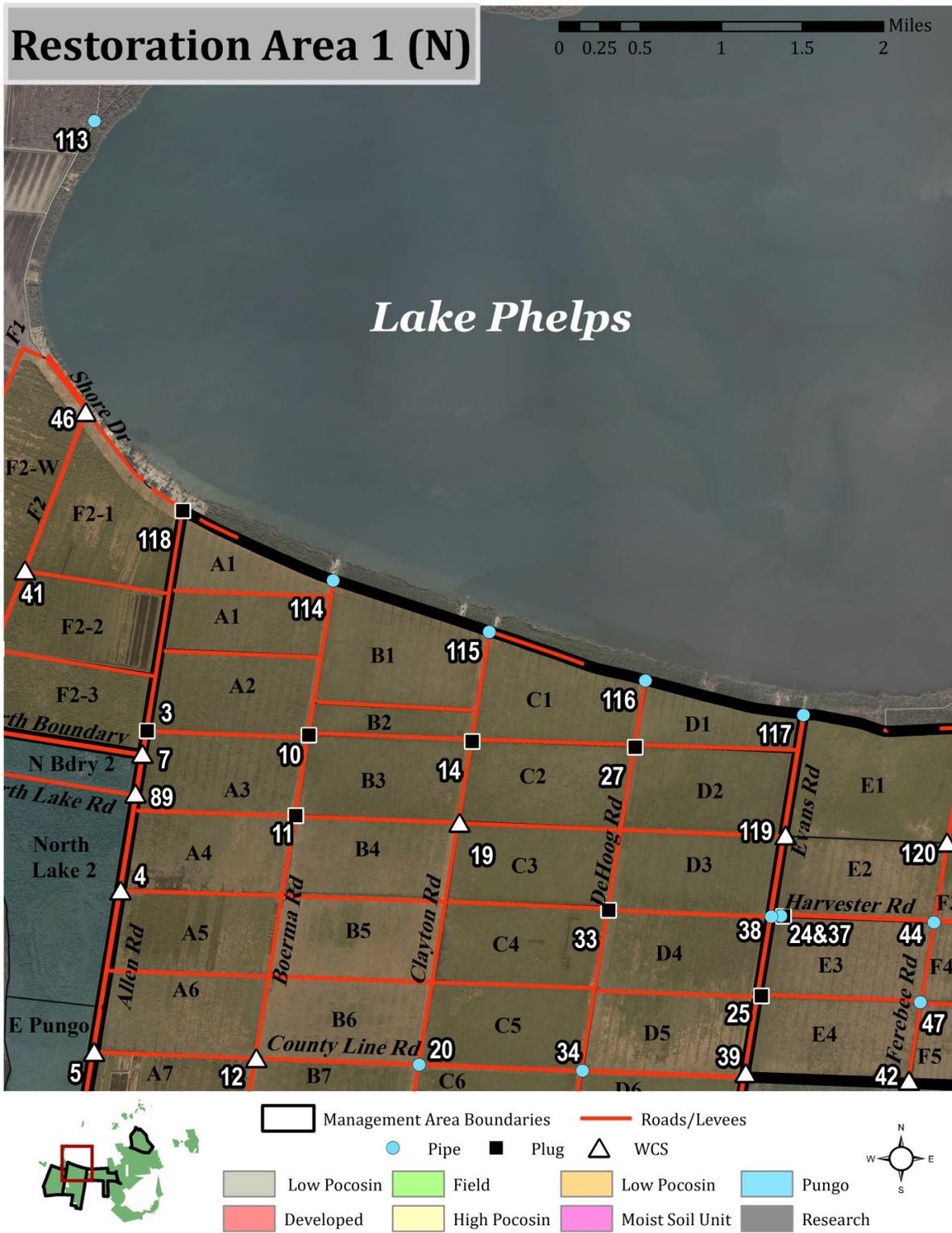
Figure E-2: Water management infrastructure within Restoration Area 1 (north) of Pocosin Lakes NWR.
