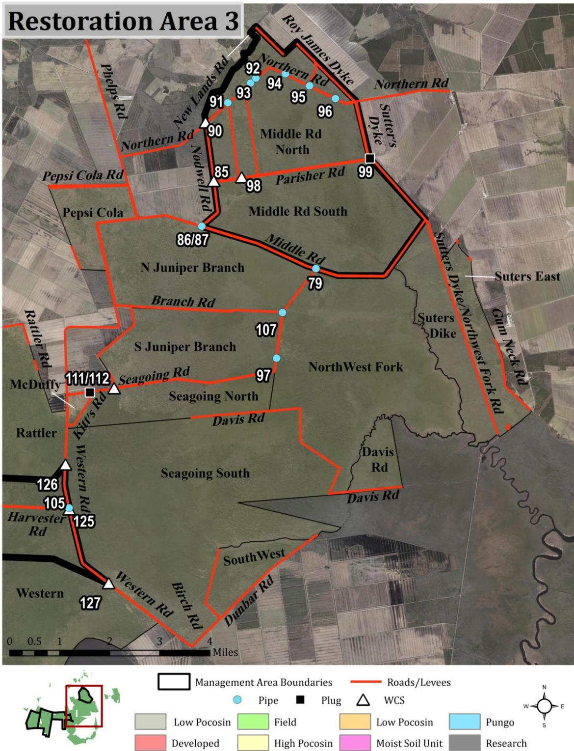
Figure E-5: Water management infrastructure within Restoration Area 3 of Pocosin Lakes NWR.
