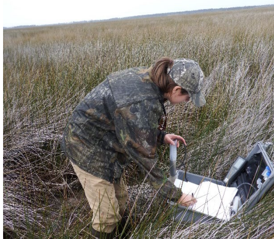
Figure 3.3. Photo of field personnel taking soil porewater salinity measurements in the field.
