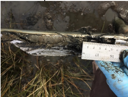
Figure 3.2. A photo of a soil core measurement. The core is taken with a McCauley corer and then the depth of soil to the recovered feldspar layer is measured in millimeters.
