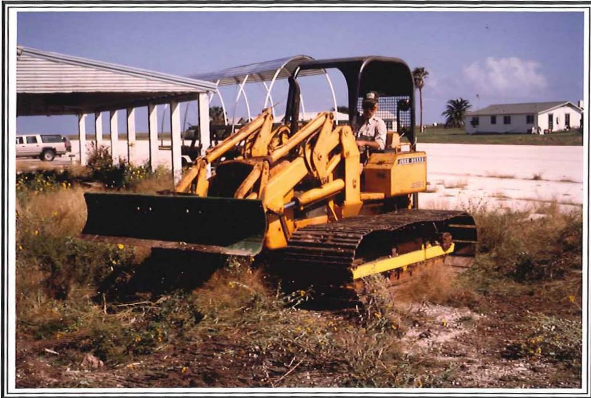
The 1973 John Deere track loader from Aransas was repaired and brought to Matagorda Island. There it was converted to a dozer for use on the levees. WM 10/98
