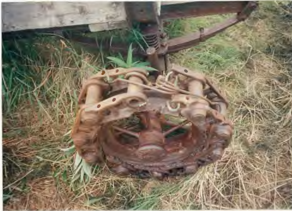
Necessity is the mother of invention. An old conibear trap was used to splice a wheel on a homemade cart. (Mike Jensen)
