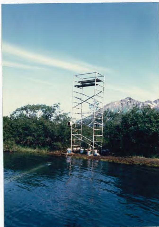
A portable counting tower set up on the east bank of the Togiak River to enumerate fish as they pass over the flash boards laid on the bottom of the river. KH, 1987.
