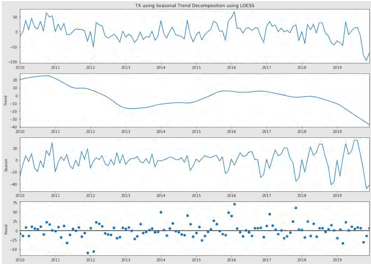
Figure A3-4. Output from our Normalized Difference Vegetation Index (NDVI) analysis for the Texas analysis unit. Plate 1: NDVI anomalies by month from 2010 through 2019. Plate 2: Seasonal trend decomposition with locally estimated scatterplot smoothing (LOESS) using a 13-month floating window. Plate 3: The variation ascribed to seasonality. Plate 4: Residuals from the model.
