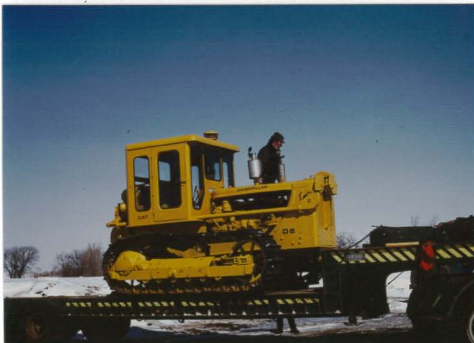
An overhauled, rejuvenated D-6 back from the Diesel Department, North Dakota State School of Science. SWB
