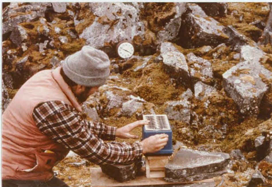
Time lapse camera being set up by Art Sowls, USFWS, Anchorage in an Auklet colony on St. Matthew. Note the solar panel for charging the camera batteries. The clock provided the time each frame was exposed. #80028 6/84 R.C.A.
