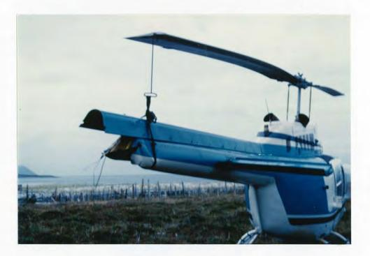
A forced landing was made after the tail rotor struck the ground during cattle herding operations on Simeonof Island in September. Parts were flown in several days later and the helicopter flew out under its own power. 9/85 T.J.E.
