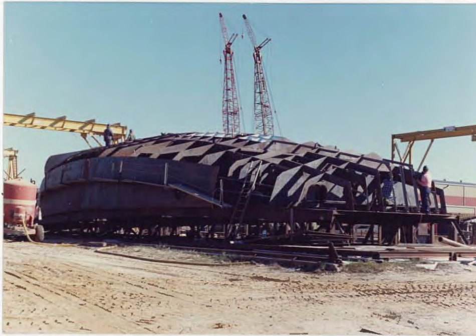
Construction of the new refuge vessel began on July 7 in Escatawpa, Mississippi. The 121 ft by 33 ft. boat will be used to support refuge operations along coastal Alaska. Basic hull framing and skin were put in place while the boat was inverted. 11/86 ADB
