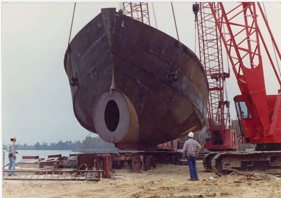
The vessel hull was righted using three cranes. The bulbous bow has yet to have the nose attached. Shortly after the bulbous bow was completed and the house attached, the boat was placed in the water. 12/86 ADB
