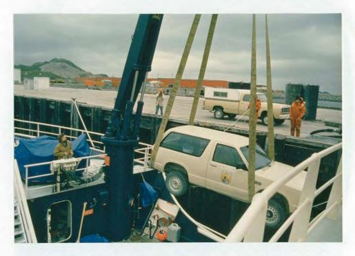
The forward crane of the <u>Tiglax</u> is rated at 16,000 pounds, capable of handling vehicles and moderate sized boats. (7/87, TJE).
