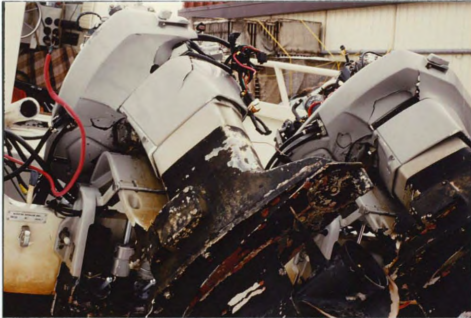
The dual 115HP outboards on the Kittiwake received major damage from the pounding surf. (EVK)
