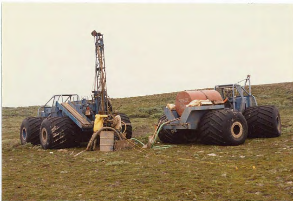
Rolligons were used to transport drilling rigs to blasting sites . . . . 20-83-GE
