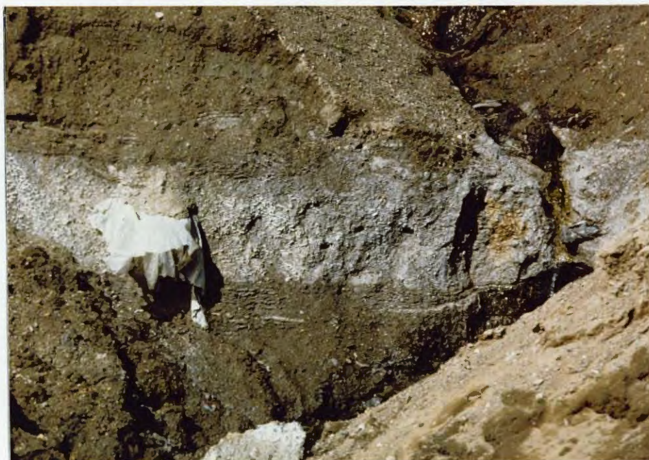
Drill mud and plastic eroding out from side of well pad. REH
