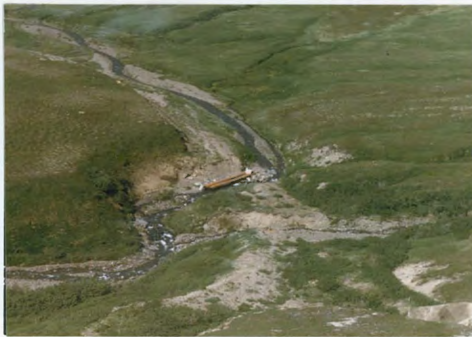
A 1959 drilling effort left a road with numerous culverts to be washed out. REH
