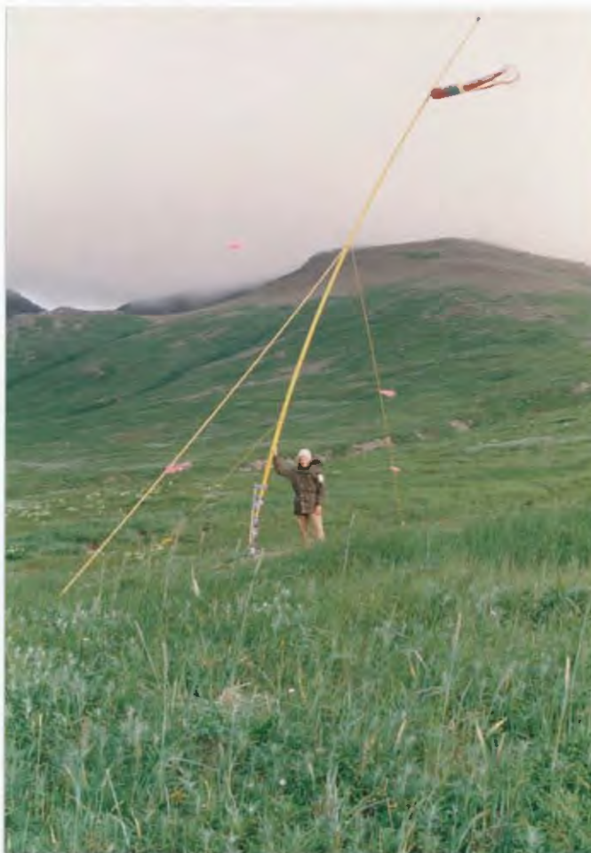
Using a hefty chain in place of a windsock provides more accurate wind speed data on the Alaska Peninsula. 7/91, BE
