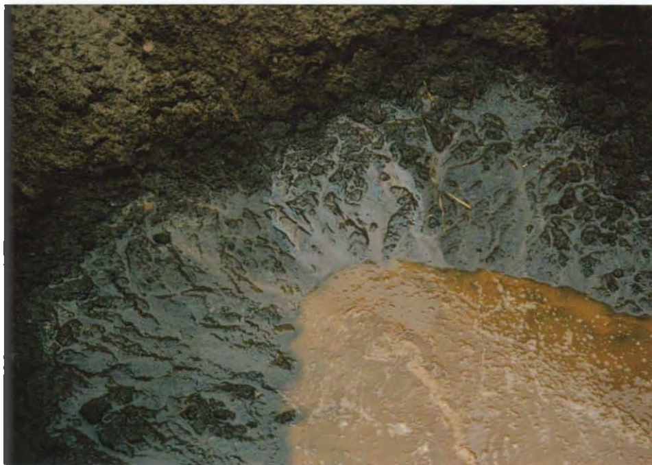
Sheen from test pit adjacent to cache demonstrates that hydrocarbons have escaped. At year's end, we were still waiting for the results of lab analysis of the numerous samples taken at the site. 6/19/92, REH
