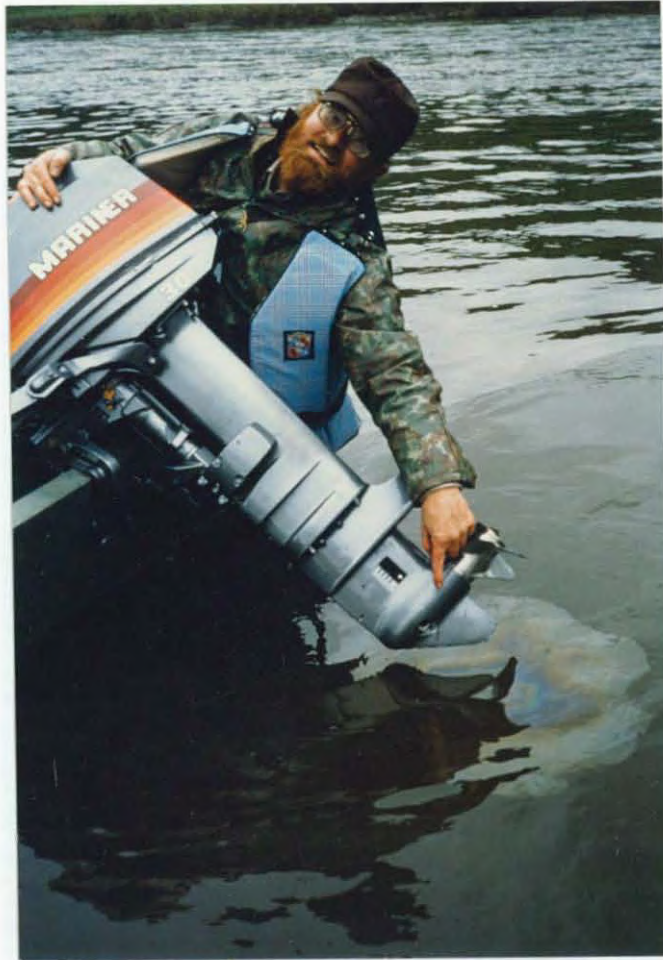
A casualty of a river trip—a new 30 hp Mariner blew the gears out both sides of the lower unit when the prop struck a rock.
