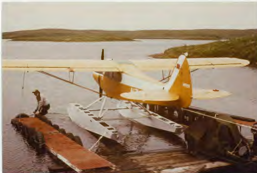
Once constructed the ramp was fitted with bumpered walkways. Weight applied beneath the walkways and ramps lowered the unit to the lake bottom.
