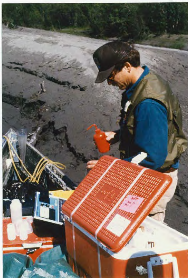
Rod Simmons of NAES conducting water analysis and collecting samples of water, sediment and tissue in an effort to detect possible contaminants from up-stream placer mines. June 1985 E.W.M.
