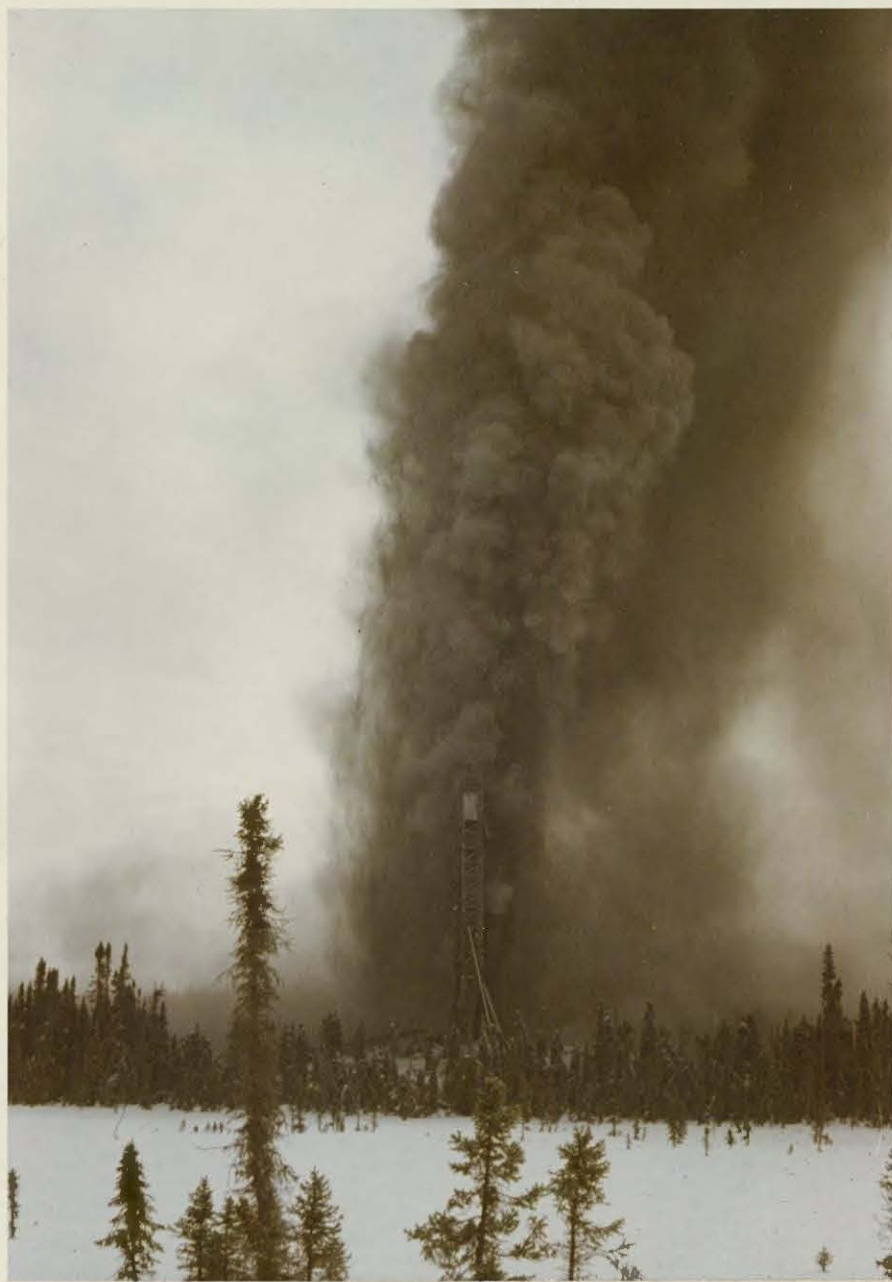
2A-61 This gas blowout occurred at the Beaver Creek well, sending rocks and silt 500 feet into the air and badly silting Beaver Creek. This is a hazard of oil operation.
