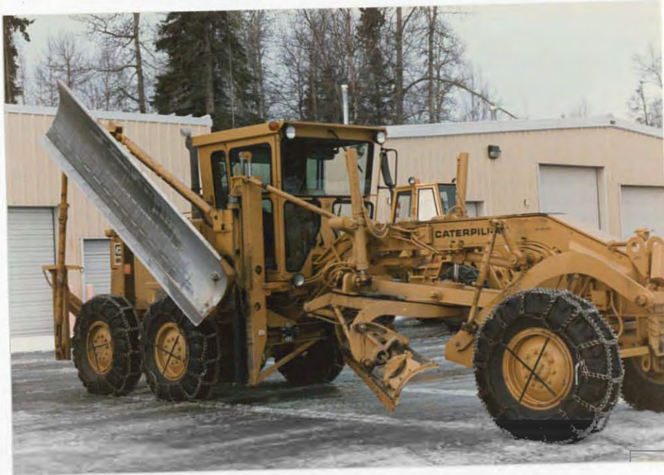
The new 12' Falls snow wing was a welcome addition to our Cat 130 grader in 1986. JF
