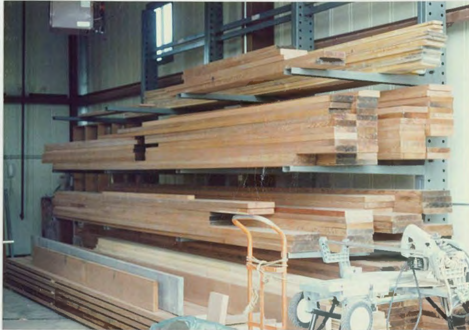
Cantilever racks greatly improved our lumber storage capability in the carpentry shop. JEF
