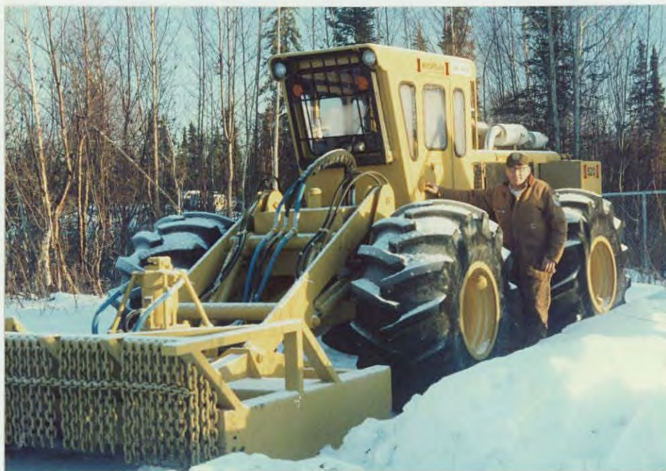
The new 520 Rotary Hydro-Ax will be used primarily for clearing fire lines as part of our fire management program.
