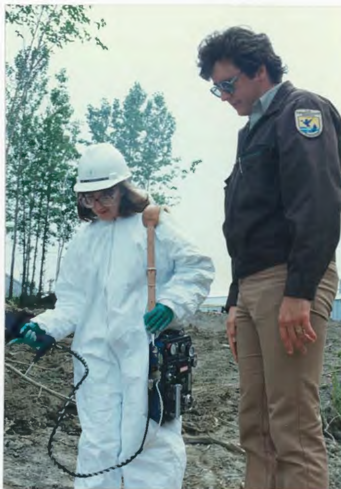
Winkelman and Ecology and Environment, Inc., Safety Specialist Karen McRoberts test for volatiles prior to release sampling for PCB's, at SRF. 7/90/JEF
