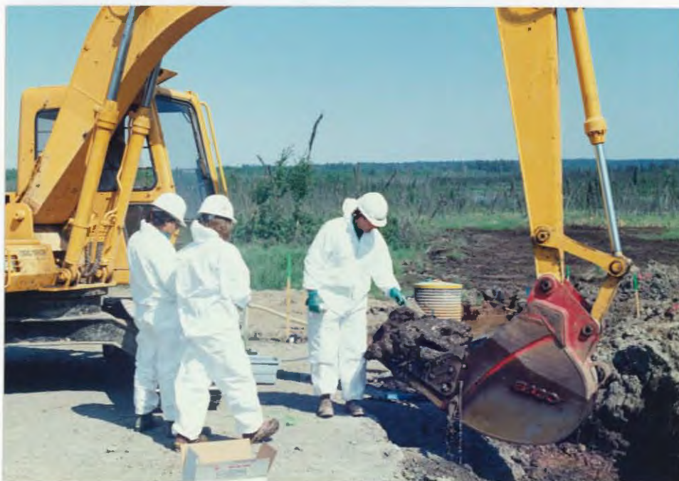
Ecology and Environment, Inc., technicians taking sub- surface soil samples for possible PCB contamination at Pipe and Supply (P&S) Yard at SRF. 7/90/JEF
