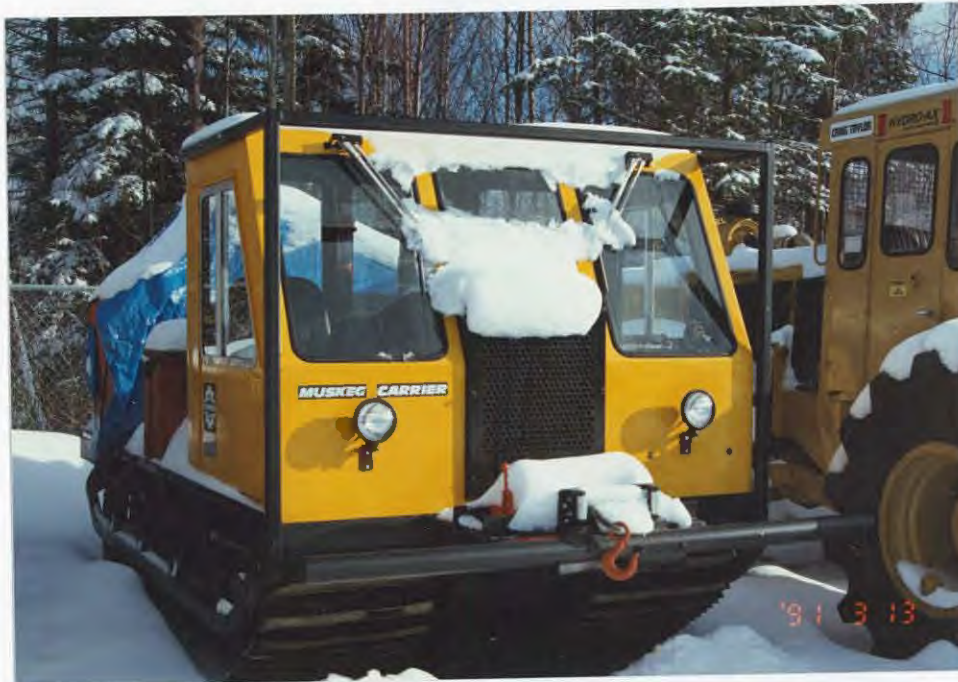
New Bombardier "Muskeg Plus" was fitted with steel bumper, hydraulic winch, reinforced cab protection and steel deck to hold 300-gallon foam tank. 1/91/JEF
