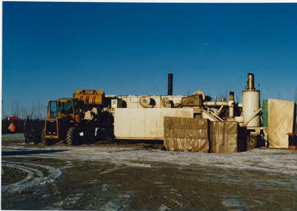
Portable Thermal Unit brought in to destroy hydrocarbon contaminated soil at Marathon Oil Co.'s BCF Production Facility. Unit was plagued by numerous problems during first field season. 9/90/JEF
