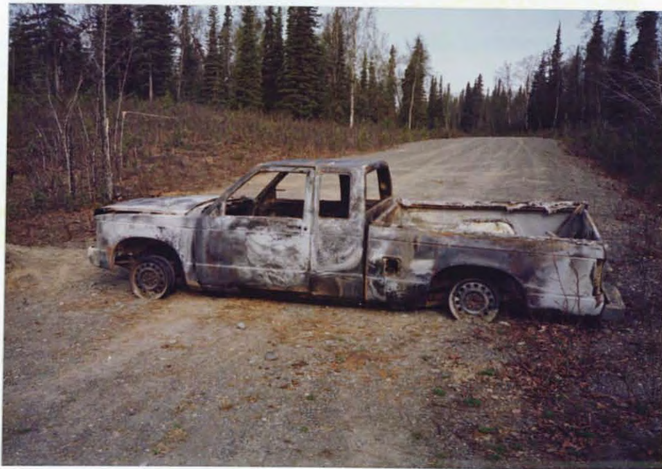
One "very well-done" S-10 Chevy pickup, the aftermath of an intensely hot fire caused by a rapidly developing electrical fire.
