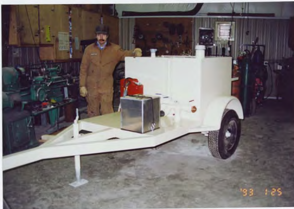
Mechanic Al O'Guinn fabricated this 200-gallon mobile, high pressure watersystem for cleaning campground restrooms and for emergency fire fighting. 92/JF
