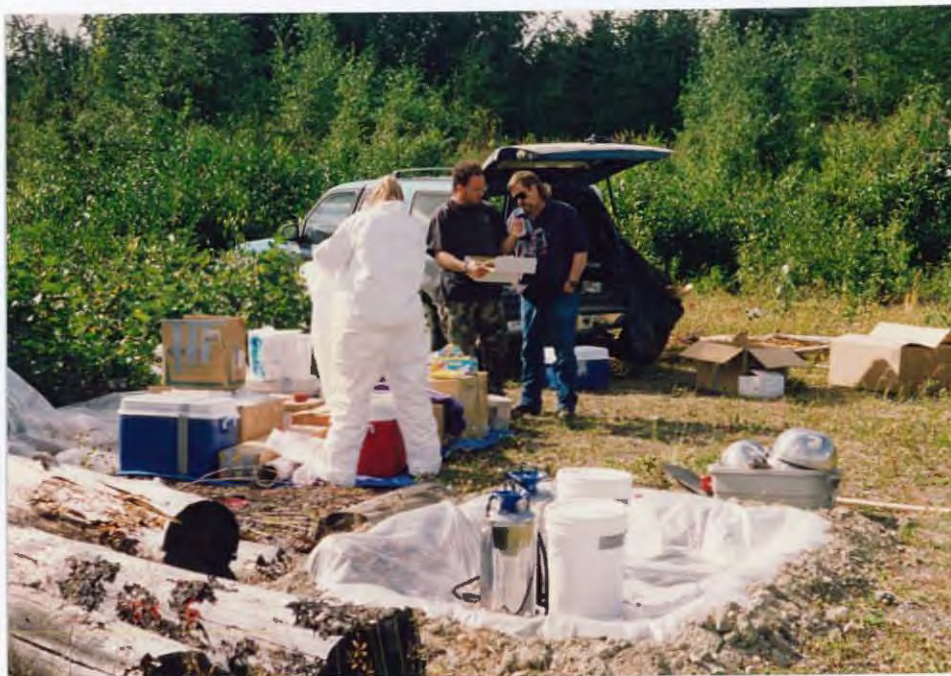
Site investigation being conducted by EBASCO Environmental, Inc. for pentachlorophenol (PCP) at the old Swan Lake #1 drill pad--site of fence post preservation activities in the late 1960's and early 1970's. 93/JF
