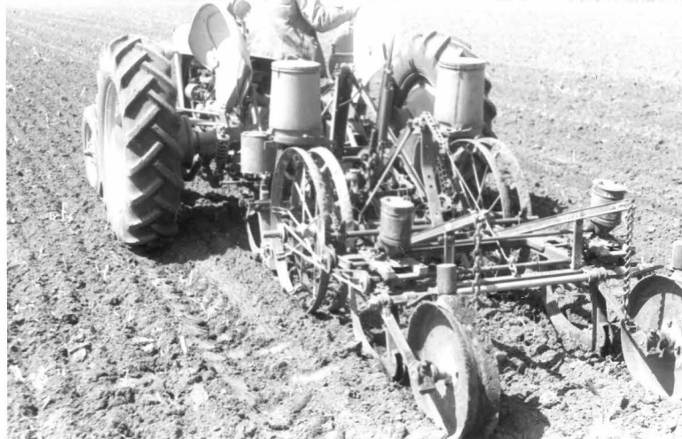
Two views of the row-crop alfalfa seeder developed at Sand Lake. Note how hydraulic lift works in lower picture; this is used for raising the machine when turning.
