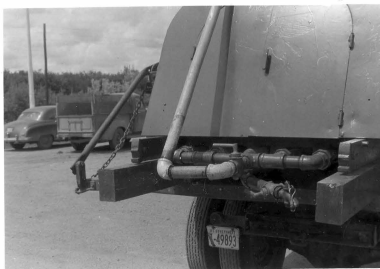
Close-up of valve arrangement on above tank. Herbicide is drawn from the lower valve.
