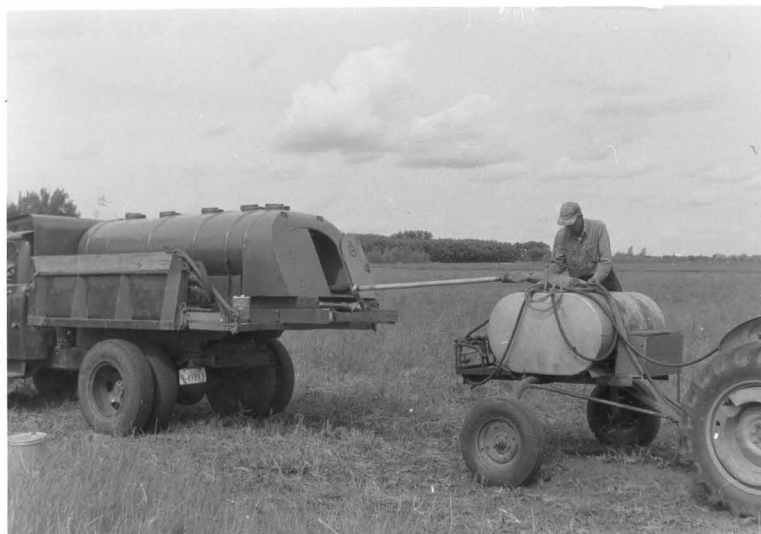
View of tank from gas truck converted for carrying water and herbicide for weed control operations. The herbicide is in the end tank. A pump seen on the left side is used for loading water. This will be helpful as a reserve during the fire season. 50-50L-811
