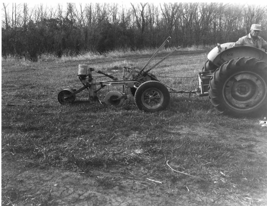
The burrow builder in action. 90% kills were made in fields poisoned at 20 foot intervals.
