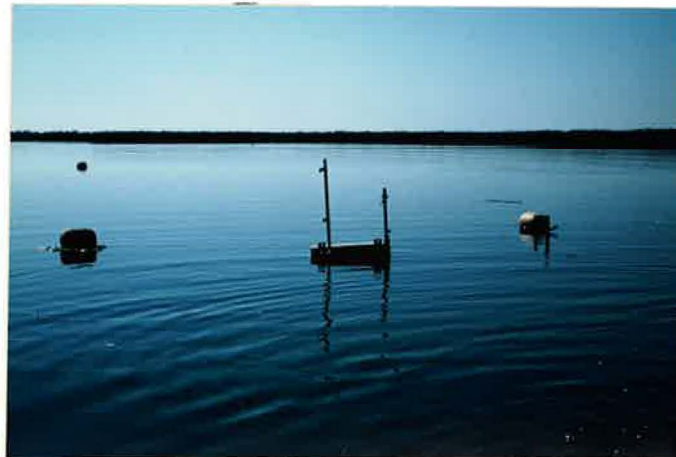
Figure 50. The main lake station sank on June 28. The pontoon welds apparently gave out after a heavy blow. The equipment was repaired and put back in operation in August. 88-JKW
