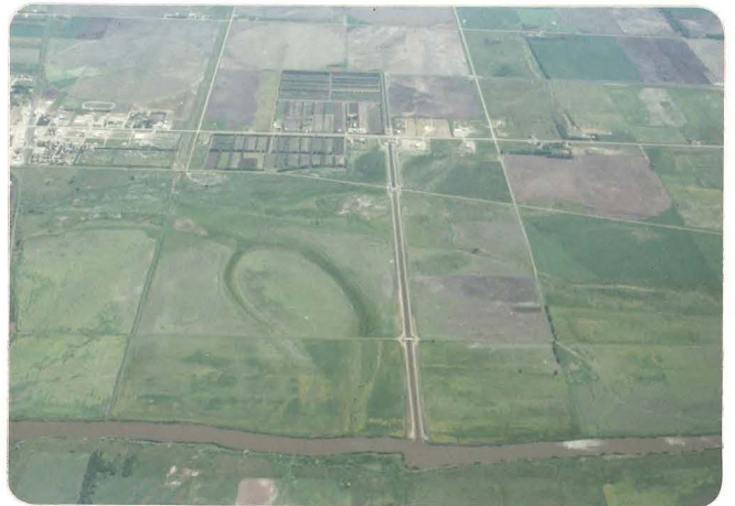
Figure 60. Stream flows are diverted from the James River (foreground) and gravity fed down the canal inlet to the Oakes Pumping Plant to provide irrigation water to agricultural lands within the 5,000 acre Oakes Test Facility (OTA). This test area prototype is located immediately upstream from Sand Lake NWR and adjacent to Dakota Lake NWR in North Dakota. Photo views east.
