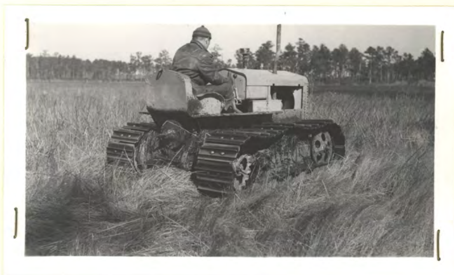
Showing use of Crawler Tractor with marsh cleats in burning of muskrat marsh. The Tractor is run around the outside of the area to be burned, making an excellent fire lane by crushing the marsh growth and allowing water to fill in the tracks.
