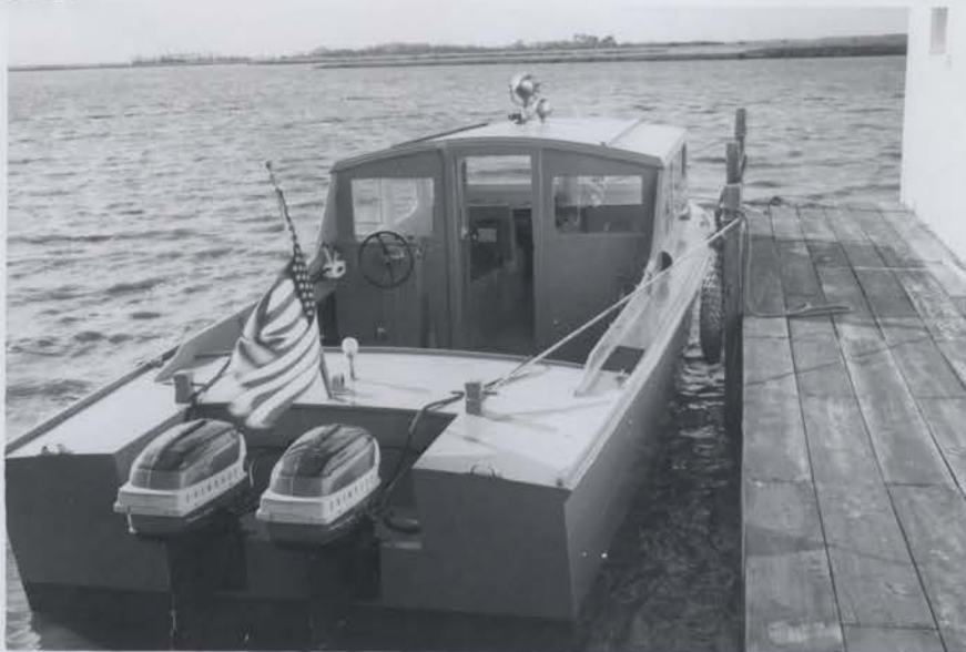
The Honker after conversion. Cockpit decking is painted with anti-skid paint. Steering wheel in cabin was removed. Windshield will be installed on top of cabin just in front of steering wheel and convertible top will be constructed at later date. Fuel lines across aft deck to be installed under deck when large fuel tanks are obtained. R-20-6, Dec., 1959.
