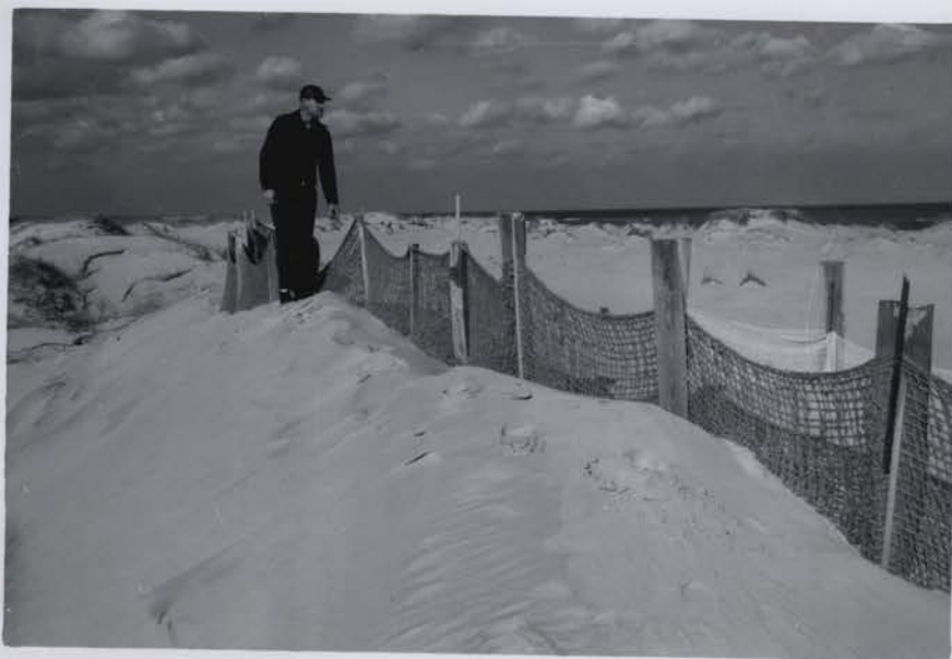
Another view of above panel showing sand piled on downwind side. R-19-1, December 29, 1959.
