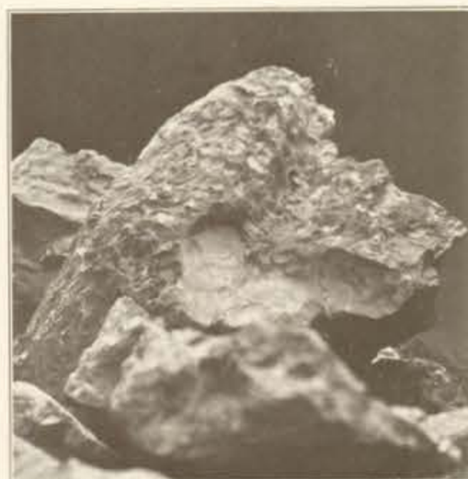
PLATE XVI.—MASS FROM TOP LAYER OF LITTLE OAK LIMESTONE WITH CHARACTERISTIC COARSE MESHWORK OF EARTHY MATERIAL ON WEATHERED SURFACE The white spots are blue limestone
