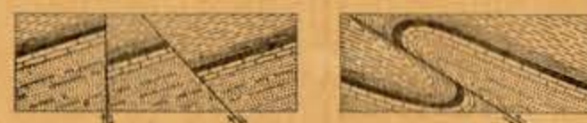
FIGURE 4.—Ideal sections of broken and bent strata, showing (a) normal faults and (b) a thrust or reverse fault.
