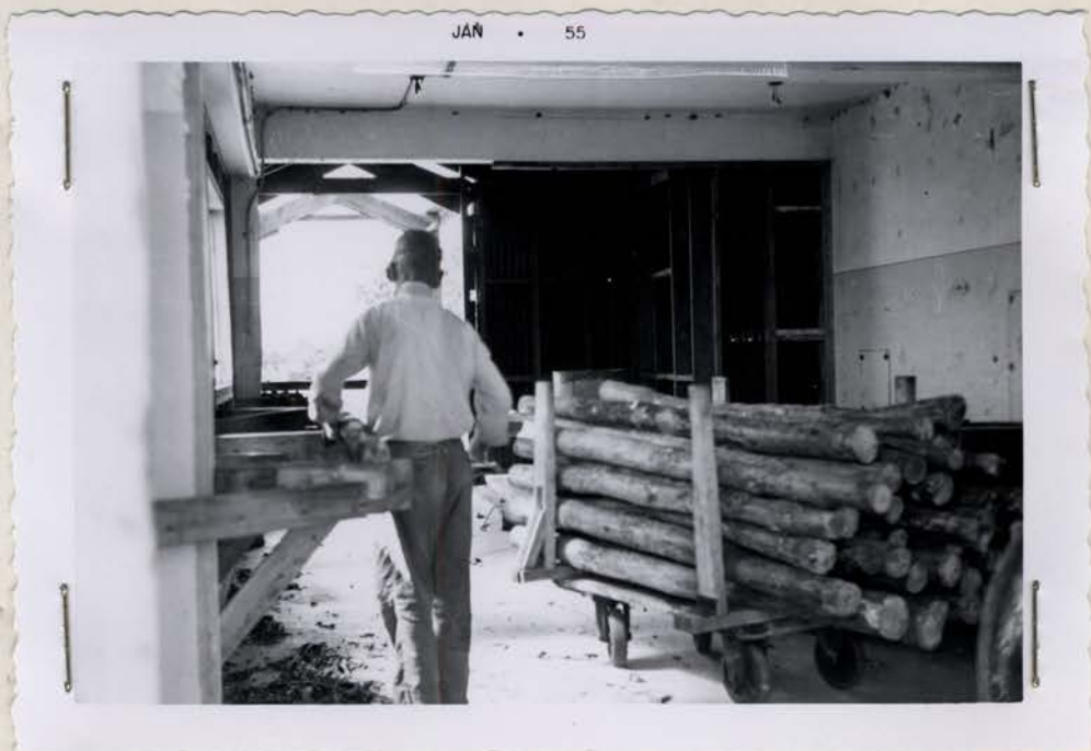
# 8. - "Knothole-Room" - where machine peeled posts are freed of protruding limb knots before air curing and then penta-treating. - Sept '54 - EEC.
