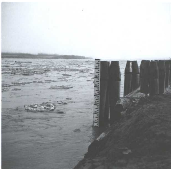
3/24/62. Missouri River gauge set by Corps of Engineers near our inlet control tube. The level is at 990.5, the day after the ice broke up. The summer navigation level is about 988. The peak of the spring rise reached 997 on March 29.
